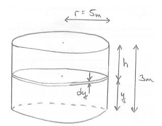
Remove water to top of the pool by a sequence of circular "thin slices" as shown. Each slice requires work
