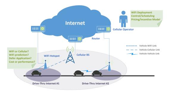
Figure 1: WiFi offloading in vehicular communication environments.
