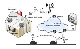
Figure 2. Two-hop communication model.
