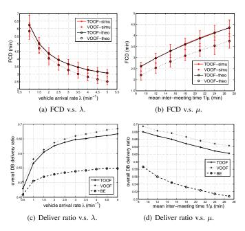
Figure 5. Performance of optimal forwarding scheme
