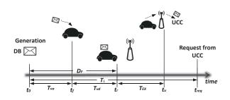
Figure 3. An illustration of time durations in the analysis.
