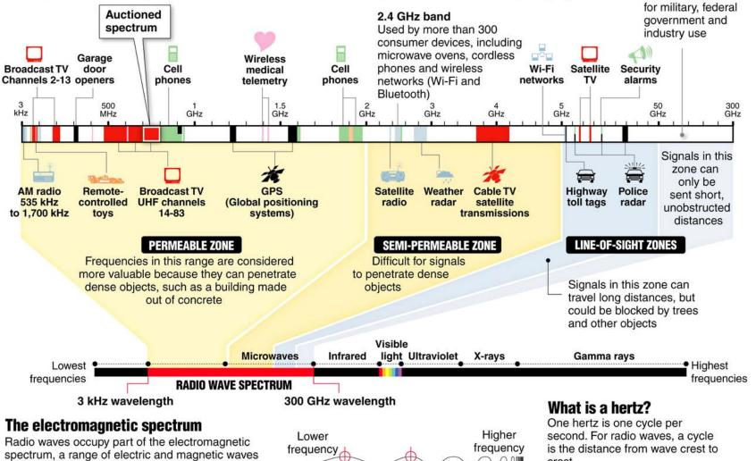
spectrum, a range of electric and magnetic waves of different lengths that travel at the speed of light; other parts of the spectrum include visible light and x-rays; the shortest wavelengths have the highest frequency, measured in hertz
